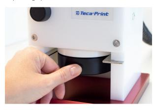
By pressing the start button, the cup housing is pushed downwards and separated from the ring blade.
