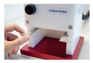
Next the clean ink cup is pushed onto the stripper plate as far as possible, with the open side of the ink cup facing up.
